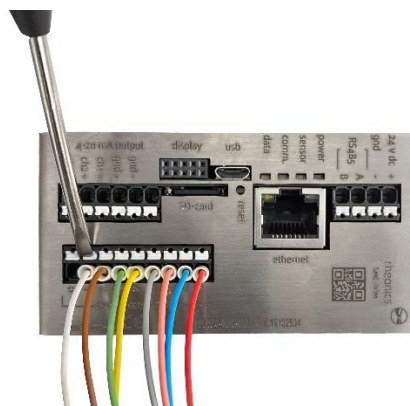
Figure 7: Disconnecting a wire from SME.
